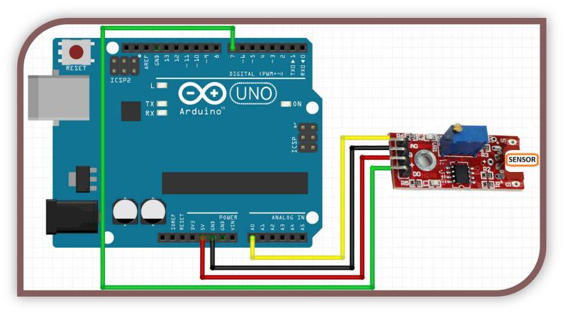
In this configuration we use "analogRead(A0)" to get the analog value, and to get the digital value we do a "digitalRead(7)". Remember to gently turn the screw in the top of the blue variable resistor to adjust the sensitivity of the digital output.
